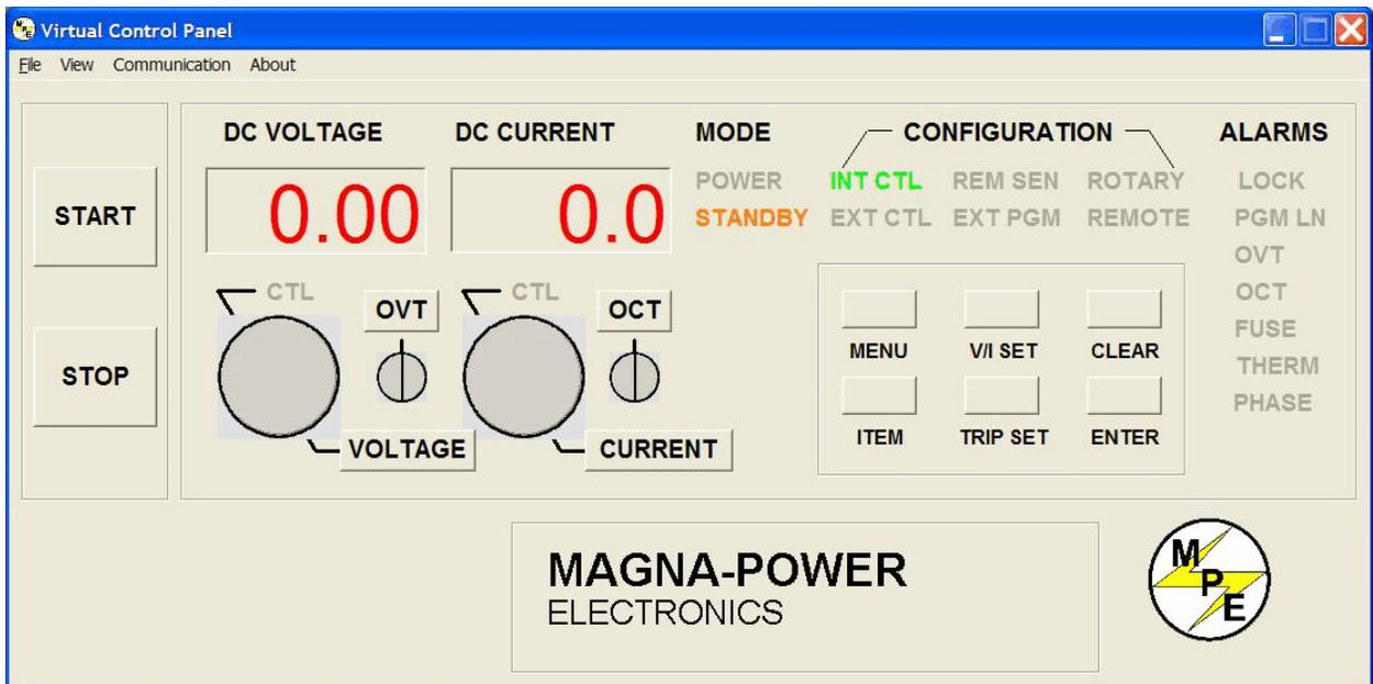
Figure 5.5 Virtual Control Panel for A Version models
