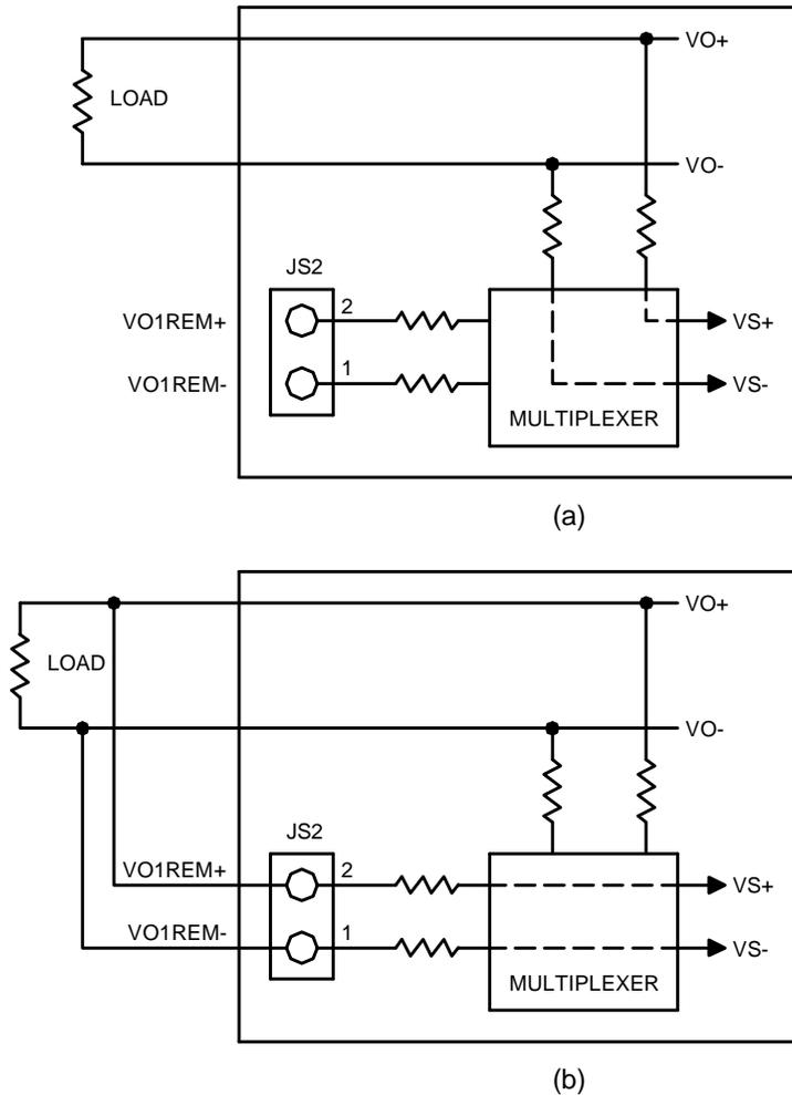
Figure 3.25 (a) Local and (b) remote sensing
