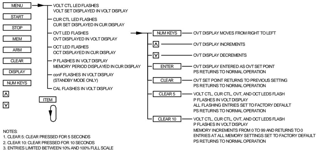
Figure 3.4 Set over voltage trip at memory displayed
