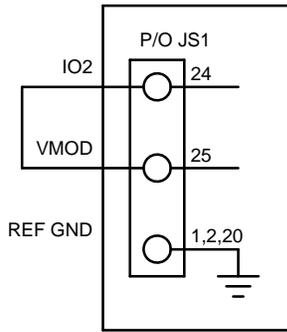
Figure 8.2 Leadless remote sensing
