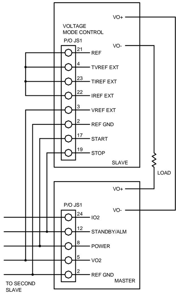
Figure 3.31 Master/slave series connection
