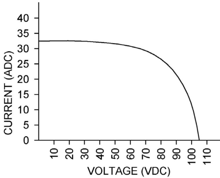
Figure 8.3 IV characteristics for a typical photovoltaic array
