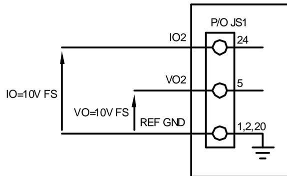
Figure 3.27 Monitoring output (a) voltage and (b) current
