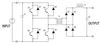
Figure 1. Voltage-Fed Converter
