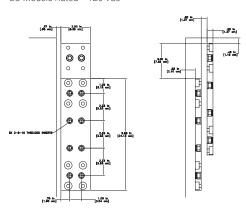
**DC Output Bus** 8U Models Rated 125 Vdc to 1000 Vdc
