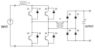
Figure 2. Current-Fed Converter
