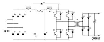
Figure 3. Rectifier, chopper, and current-fed converter
