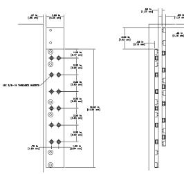
**DC Output Bus** 12U Models Rated 125 Vdc to 1000 Vdc
