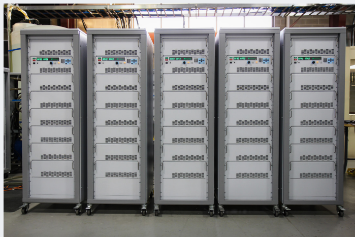
Five 100 kW WRx Series MagnaLOADs in digital master-slave parallel, performing as a single 500 kW system with measurement aggregation
