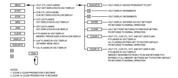
Figure 3.2 Set voltage output at memory displayed
