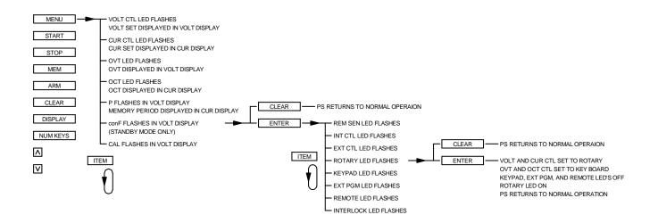
Figure 3.10 Set rotary input
