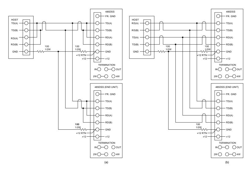
Figure D.1 RS485 (a) 2-wire and (b) 4-wire connections
