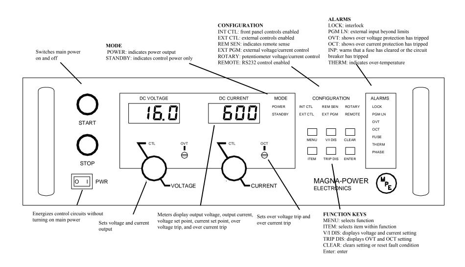
Figure 2.2 MTA Series controls and indicators
