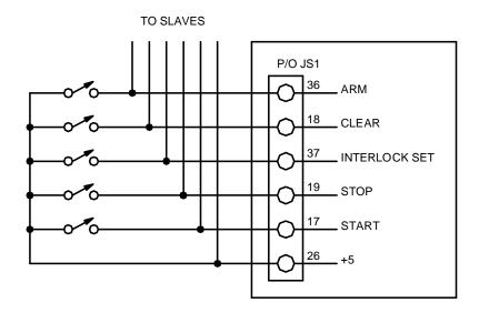
Figure 3.28 Digital input control lines
