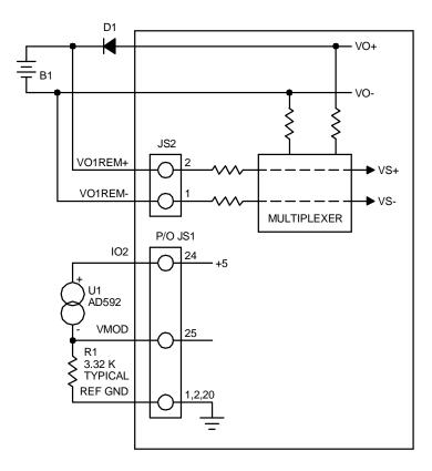
Figure 8.4 Battery charger with temperature compensation
