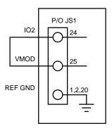
Figure 8.2 Leadless remote sensing
