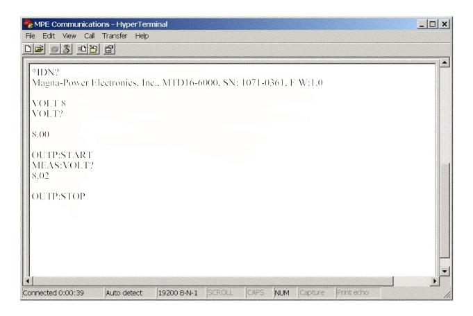
Figure 4.1 RS232 Communications using Microsoft Windows (tm) HyperTerminal
