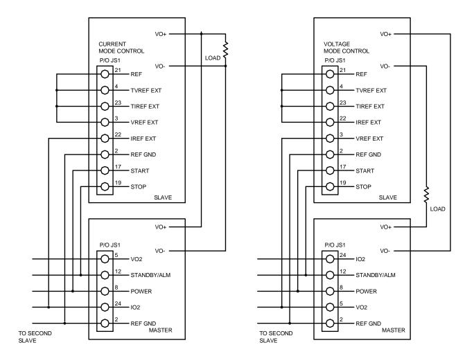
Figure 3.30 Master/slave parallel connection
