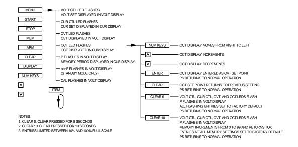
Figure 3.5 Set over current trip at memory displayed
