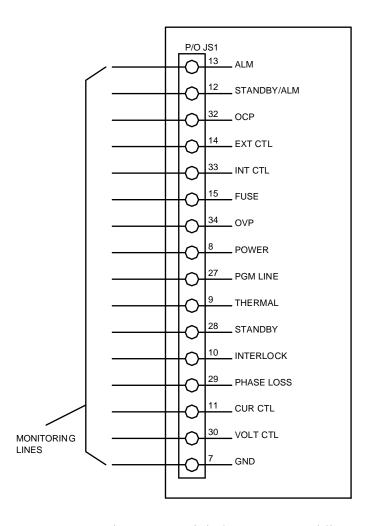
Figure 3.29 Digital output control lines
