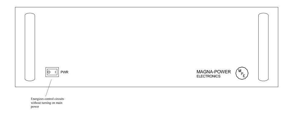
Figure 2.3 MTC Series controls and indicators
