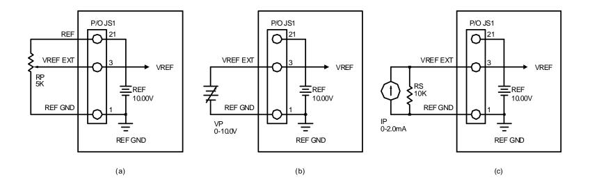
Figure 3.26 External (a) resistive, (b) voltage, and © current programming
