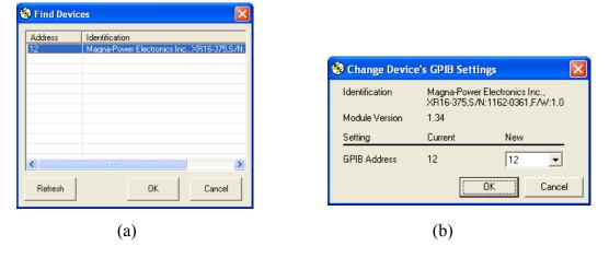
Figure 5.3 Find devices and (b) change device's GPIB settings
