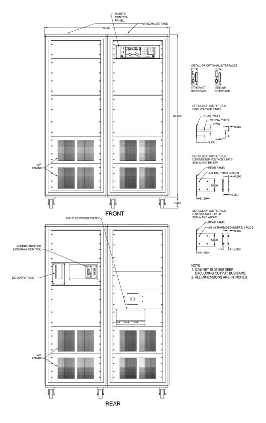
Figure 1.2 MT Series package drawing for 100 kW and 150 kW models with D Version front panel
